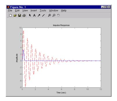
**Comparison of Open- and Closed-Loop Impulse Response**
