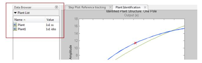
You can define the model structure and initialize the model parameter values using one of these plants. To do so, in the **Plant Identification** tab, in the **Structure** menu, select the linear plant model you want to use for structure an initialization.
