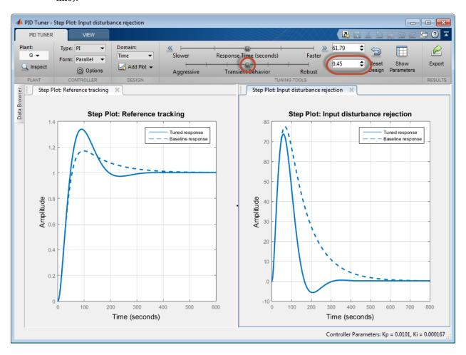
Lowering the transient-behavior coefficient to 0.45 speeds up disturbance rejection, but also increases overshoot in the reference-tracking response.
