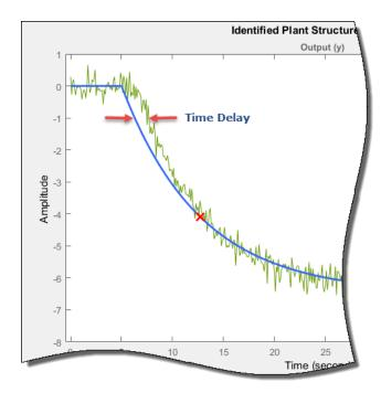
To add a transport delay to the estimated plant model, in the **Plant Structure** section, check **Delay**. A vertical line appears on the plot, indicating the current value of the delay. Drag the line left or right to change the delay, and make further adjustments to the system response by dragging the red x.
