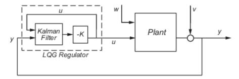
The plant in this model experiences disturbances (process noise) w and is driven by controls u. The regulator relies on the noisy measurements y to generate these controls. The plant state and measurement equations take the form of
