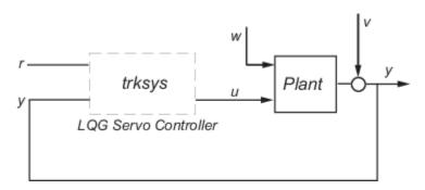
The plant has three states (x), two control inputs (u), two random inputs (w), one output (y), measurement noise for the output (v), and the following state and measurement equations:
