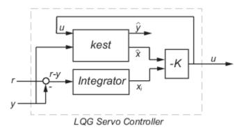
The servo controller has the following state-space equations:
