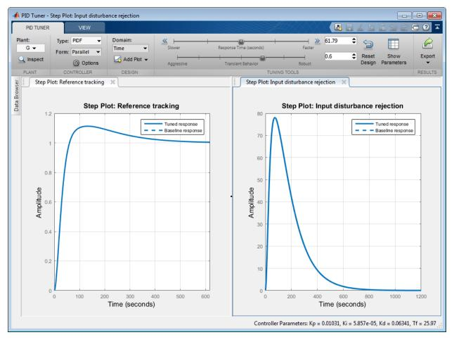
Change the **PID Tuner** design focus to favor reference tracking without changing the response time or the transient-behavior coefficient. To do so, click **Options**, and in the **Focus** menu, select Reference tracking.
