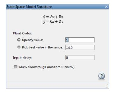
Use the dialog box to specify model order, delay and feedthrough characteristics. If you are unsure about the order, select **Pick best value in the range**, and enter a range of orders. In this case, when you click **Estimate** in the **Plant Estimation** tab, the software displays a bar chart of Hankel singular values. Choose a model order equal to the number of Hankel singular values that make significant contributions to the system dynamics.
