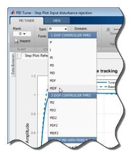
**PID Tuner** automatically designs a controller of the new type, PIDF. Move the **Transient Behavior** slider to set the coefficient back to 0.6.
