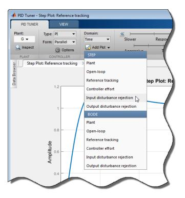
PID Tuner tiles the disturbance-rejection plot side by side with the reference-tracking plot.
