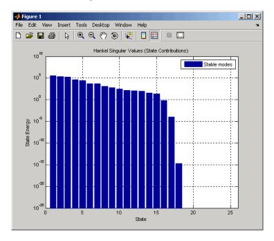
Discarding the last 8 states (associated with the 8 smallest Hankel singular values) should have little impact on the error in the resulting 17th order system.
